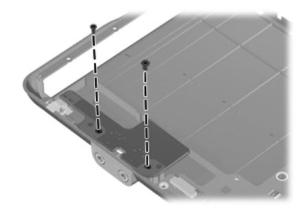
Where used: 2 screws that secure the audio board to the base enclosure
